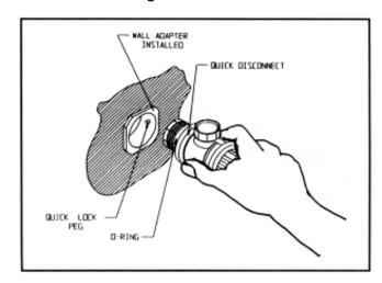
5. Take the Wall Fitting and Twist Lock the Wall Fitting into the Wall Adapter 1/4 turn; to a snug fit. Once the Wall Adapter is secure you can now twist lock and unlock to remove Wall Fitting with ease from the Wall Adapter.
